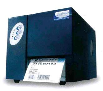
The Challenger® Series symbolizes Performance, Value and Reliability. These printers are equipped with a 32 bit Motorola RISC processor that ensures a fast first label output and serialized data printing. The entire series features a robust all metal construction designed to withstand adverse operating conditions making them ideal for heavy-duty industrial applications.
